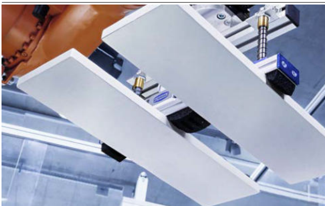
Area gripper FXP-60 when handling furniture panels
