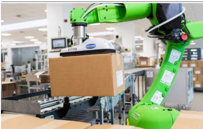
Gripping system FXCB with sealing foam for handling cardboard boxes
