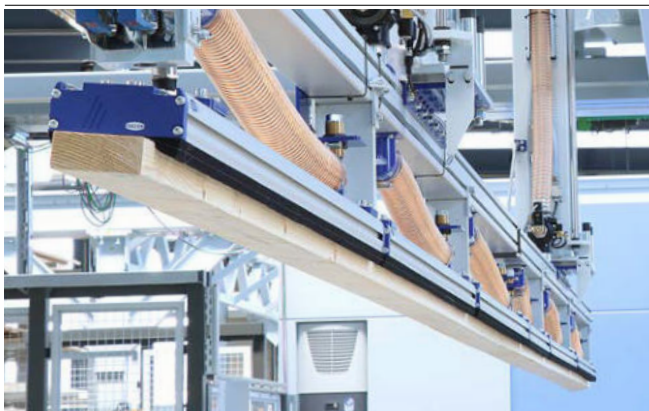
Gripping system FMP for layer-wise stacking of construction wood
