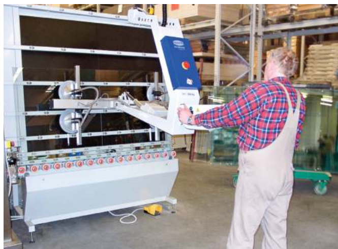
Vacuum lifting device VacuMaster Comfort for turning a glass sheet by 180°
