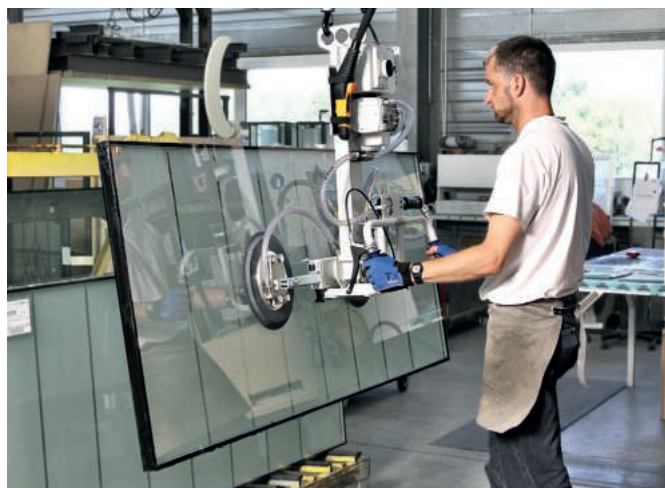
Vacuum lifting device VacuMaster Window for vertical handling of glass elements
